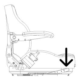
Control Handle Height: Handles are factory installed in the highest position. To lower, unscrew knob and adjust handle and hardware to desired position.
