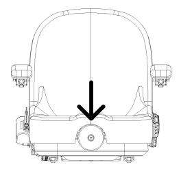
Long Travel Suspension: Lift seat using the rear latch, then adjust console suspension using the knob behind the battery.
