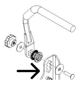
Control Handle Angle: Loosen knob and adjust handle forward or rearward to desired angle.
