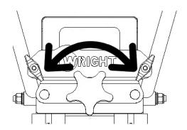
• Seat Position: Remove all weight from seat then press orange latch towards seat to adjust seat forwards or rearwards.
