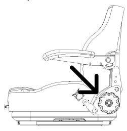
Seat Suspension: Use the dial at the front of the seat to adjust the stiffness of the in seat suspension
