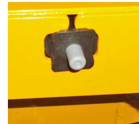
Seat up Switch Located under the seat, right side P/N 52410006 / DP black
