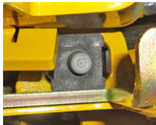
Control Levers Switch Located below each handle assy. P/N 52410006 / DP Black
