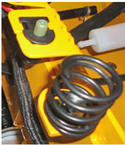
Seat Switch Located under the seat P/N 52410003 / SP black
