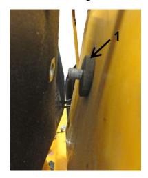
4. Attach 9" vent line to vent valve and route in-between upright and fuel tank.
