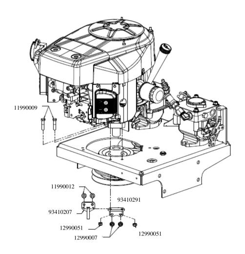
New bolt in clutch stop moves to the forward engine bolt mounting location and utilizes the second stop location on the clutch bell housing. Orientation of the clutch bell housing stays the same.
