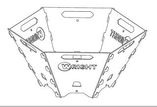
6. Place the fire pit bottom plate into the bottom of the hexagon to complete the fire pit.
