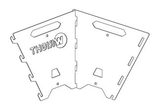
5. Continue assembly of the sides, alternating between hooked and slotted, until you have completed the hexagon.
